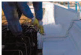
Lightened blank samples are placed on the negative and glued to each other by the heads.
